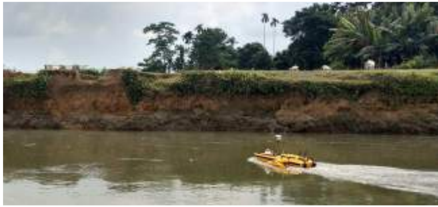
River Survey with remote controlled hydrographic survey boat
